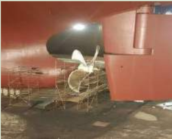
PBCF fitted on SCI VLCC- DESH UJAALA
