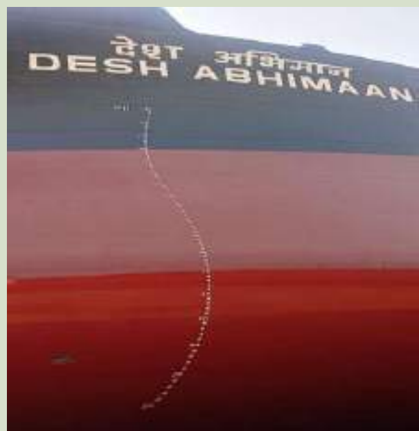
Silicon paint applied on underwater portion of SCI tanker DESH ABHIMAAN
