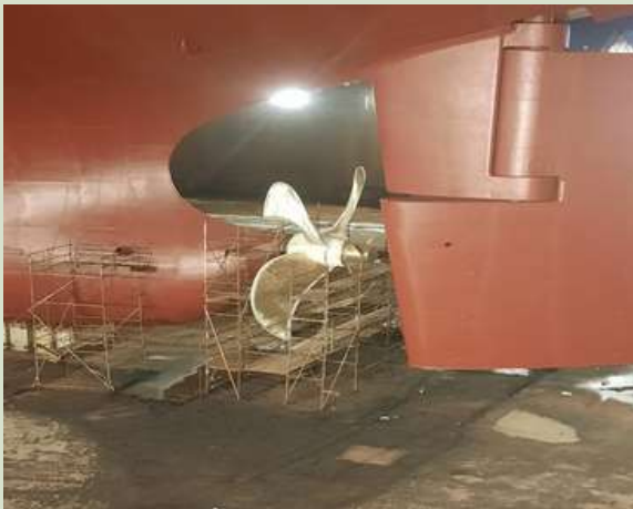
PBCF fitted on SCI VLCC- DESH UJAALA
